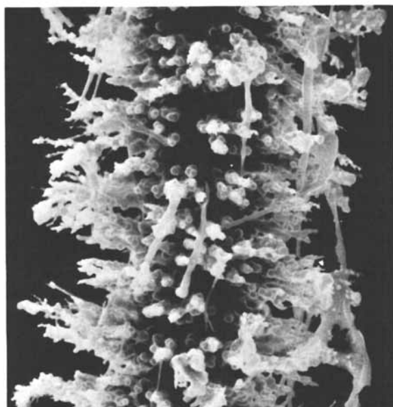
Figure 4. Electron micrograph of activated emitter to which sample has been applied by dipping emitter into a solution and allowing the solvent to air dry.
